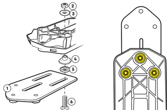
6. Apply a thin layer of sealant around the mounting holes for the front mirror on the cab (yellow marking).
